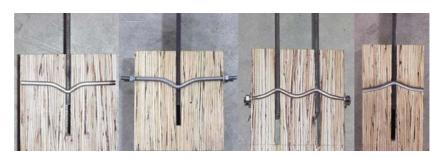
Figure 3 – Deformed Fasteners (Series D, E, F and G)
