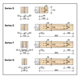
Figure 2 – Specimen Dimensions
