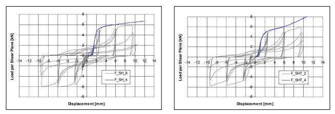
Figure 5 – Typical F\_SH and F\_SHT Cyclic and Monotonic Load-Displacement Curves
