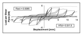
Figure 10 – E\_SH Calculated Hysteresis Curve (Calculated Monotonic Curve Shown in Grey)
